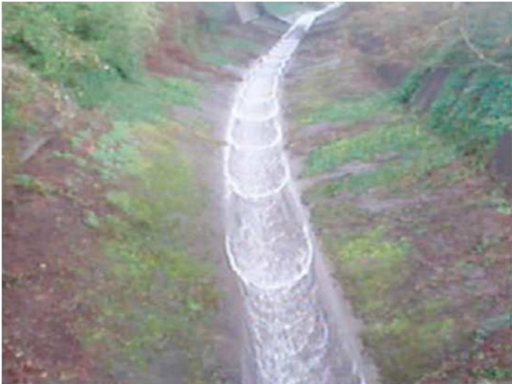
Figure 4.6: Roll waves propagating down a spillway at Lion's Bay, British Columbia. The width of the flow is about 2 m, and the water depth is about 10 cm. Photograph courtesy Neil Balmforth.
