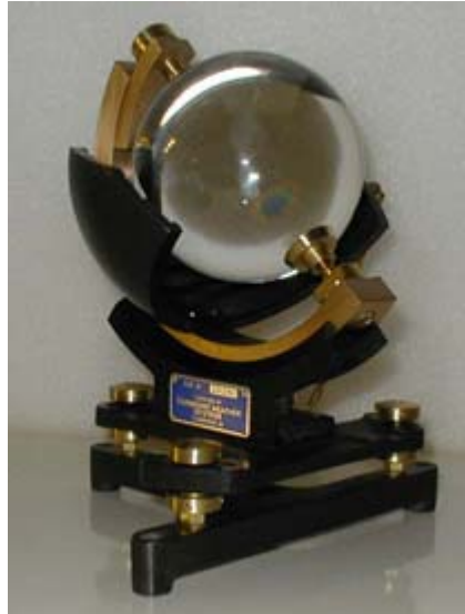
Figura 4.3- Dispositivo para achar o valor de n denominado Campbell Stokes http://www.russell-scientific.co.uk/meteorology/campbell_stokes_sunshine_recorder.html
